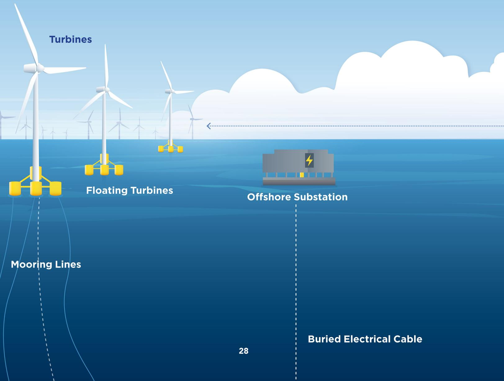
A buried transmission cable transmits the power from the floating substation to the shore, where it is connected to the existing onshore electrical grid.
