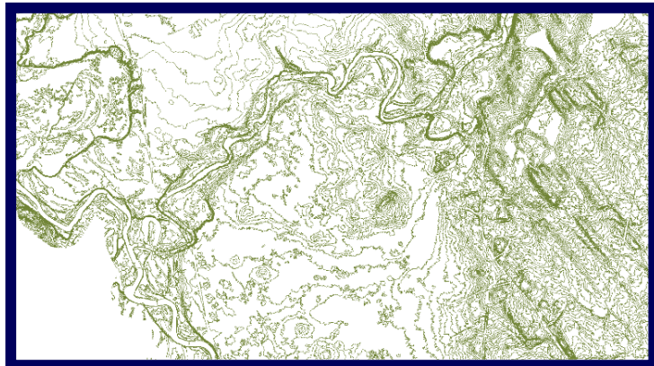
Figure 6. Two-foot contours – A derivative product developed from LiDAR.
