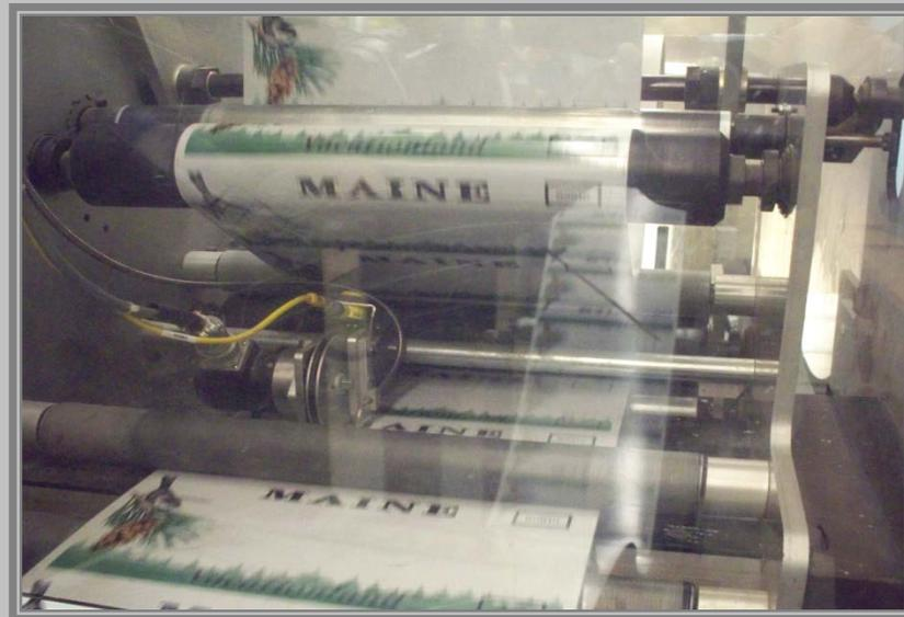
The Passenger Plate design that depicts Maine's State bird, the Chickadee, is being applied to the aluminum and will continue on its way to be cut into license plate blanks.
