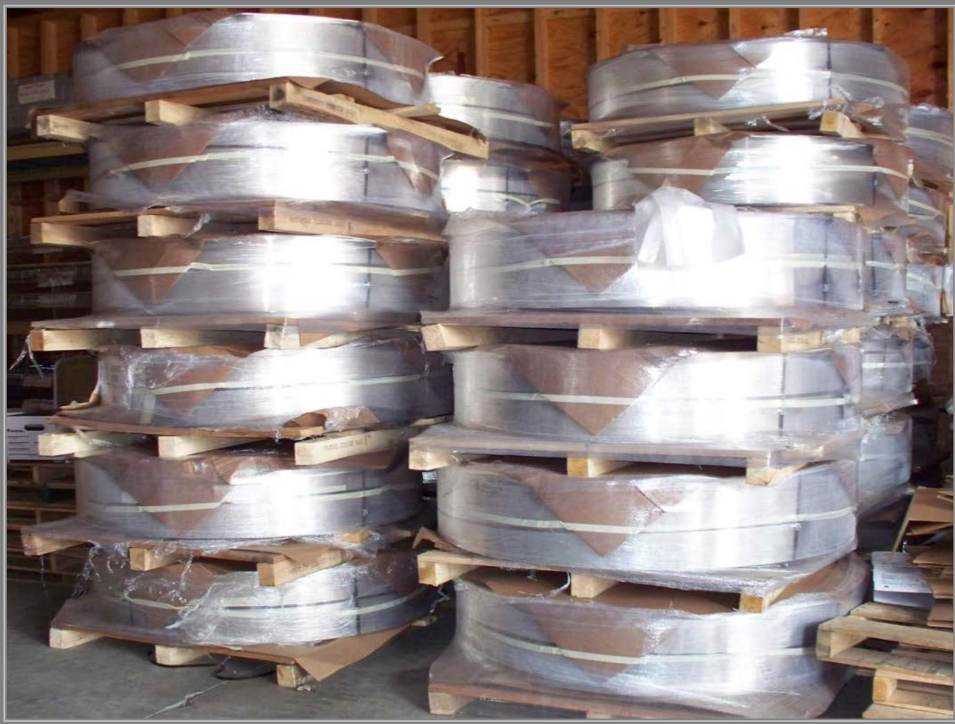
**Rolls of aluminum also are stored in the Warehouse. Each roll of aluminum weighs between 1,200 and 2,200 lbs.**
