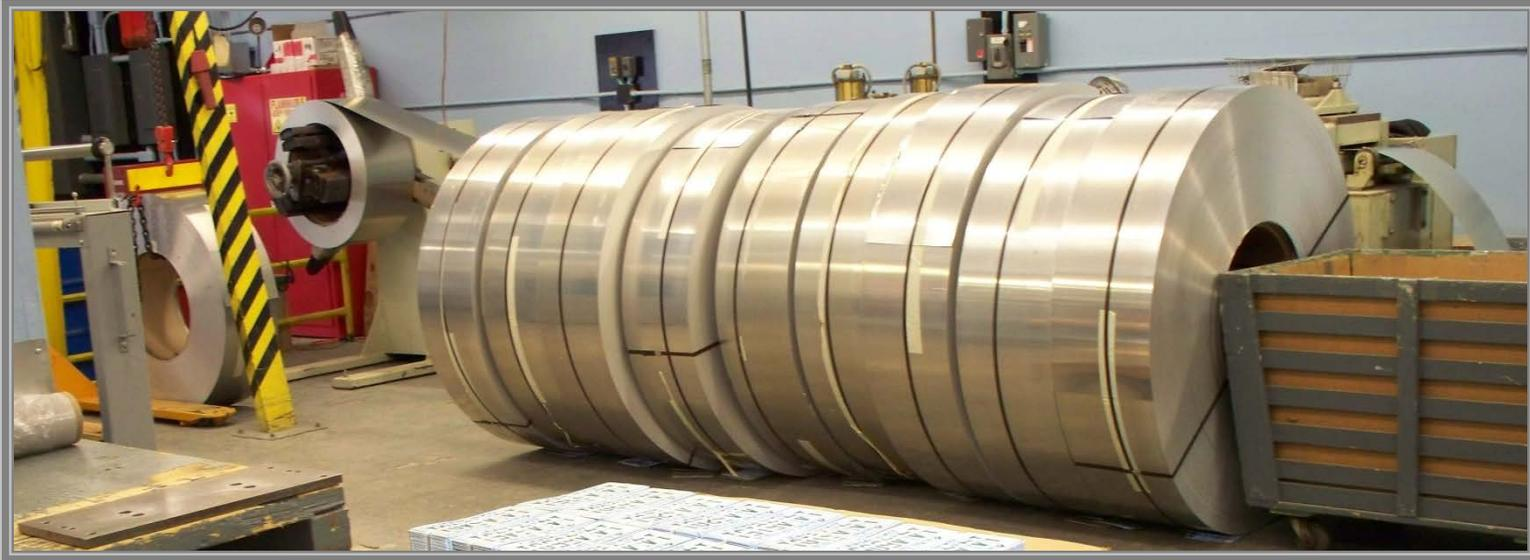
Upon entering the Plate Shop, rolls of aluminum are in view and standing upright ready for processing. Each roll of aluminum weighs between 1,200 and 2,200 lbs.
