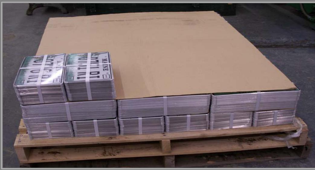
A full skid pallet has 5,000 pairs or 10,000 plates stacked and ready for shipping and each full pallet weighs 2,500 pounds. (Four plates equal a pound).
