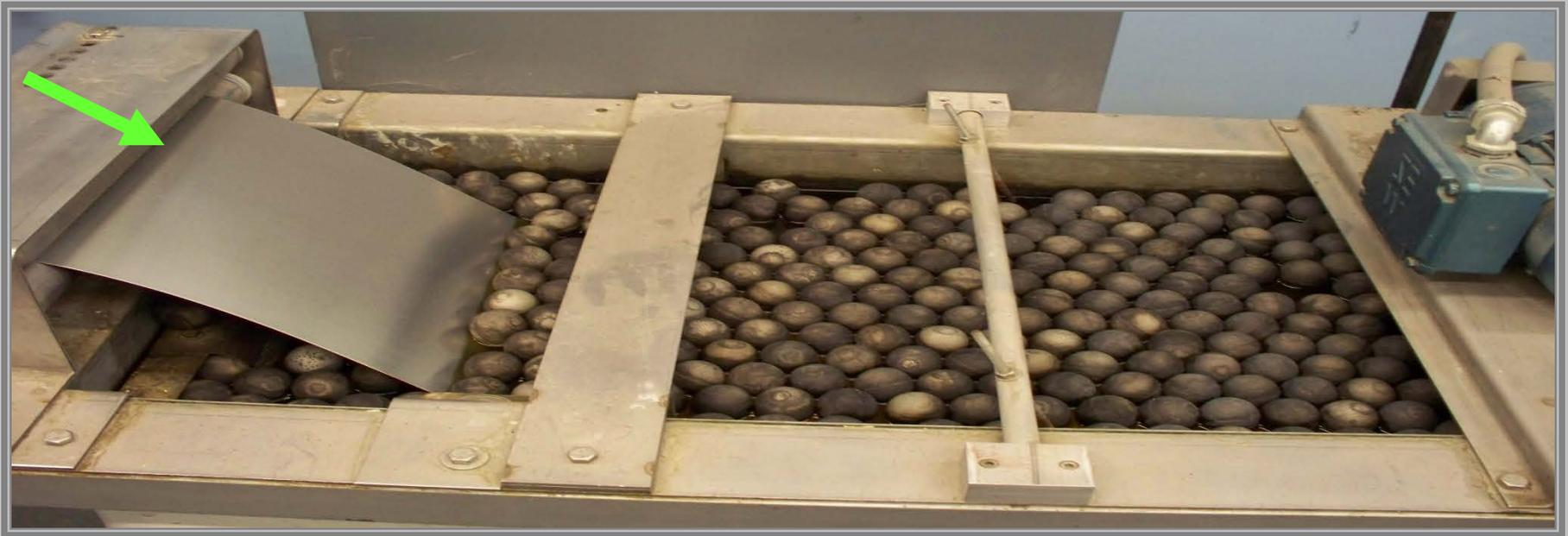
As the aluminum unrolls, it is submerged in a pre-heated (350 degree) tub of hot water. Hollow (ping-pong type) balls float on the surface of the water and assists with holding the metal under water to maintain the necessary heat and moisture to soften the aluminum. The aluminum exits through two rollers that compress the metal to remove the water as the metal is guided through the roller slot. An offset fan waves air over the top of the aluminum to assist with the drying process.
