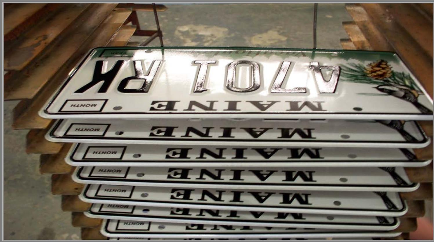
Once the rack returns from the oven, each plate is removed, checked, shrink wrapped as pairs, and strapped into 50 plate bundles or 25 pairs. The bundles are stacked on a skid pallet. (Single plates, such as trailers and motorcycles, are not shrink-wrapped, just strapped in bundles and stacked on skid pallets).
