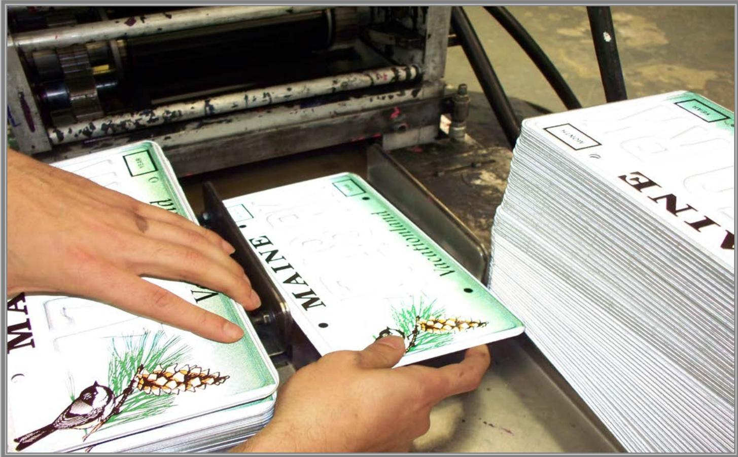
Each plate is individually placed in a slot that is belt driven through the inking machine and runs over the conveyor rollers.
