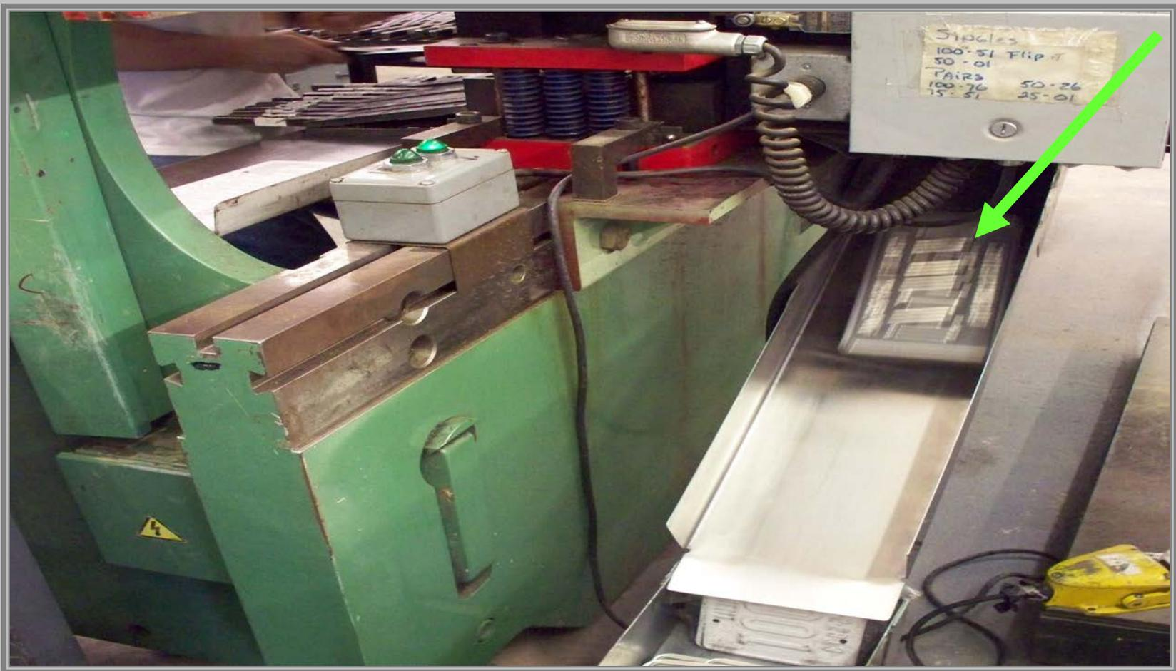
The third operator catches the embossed plate from the exit tray and stacks the plates, preparing them for inking.
