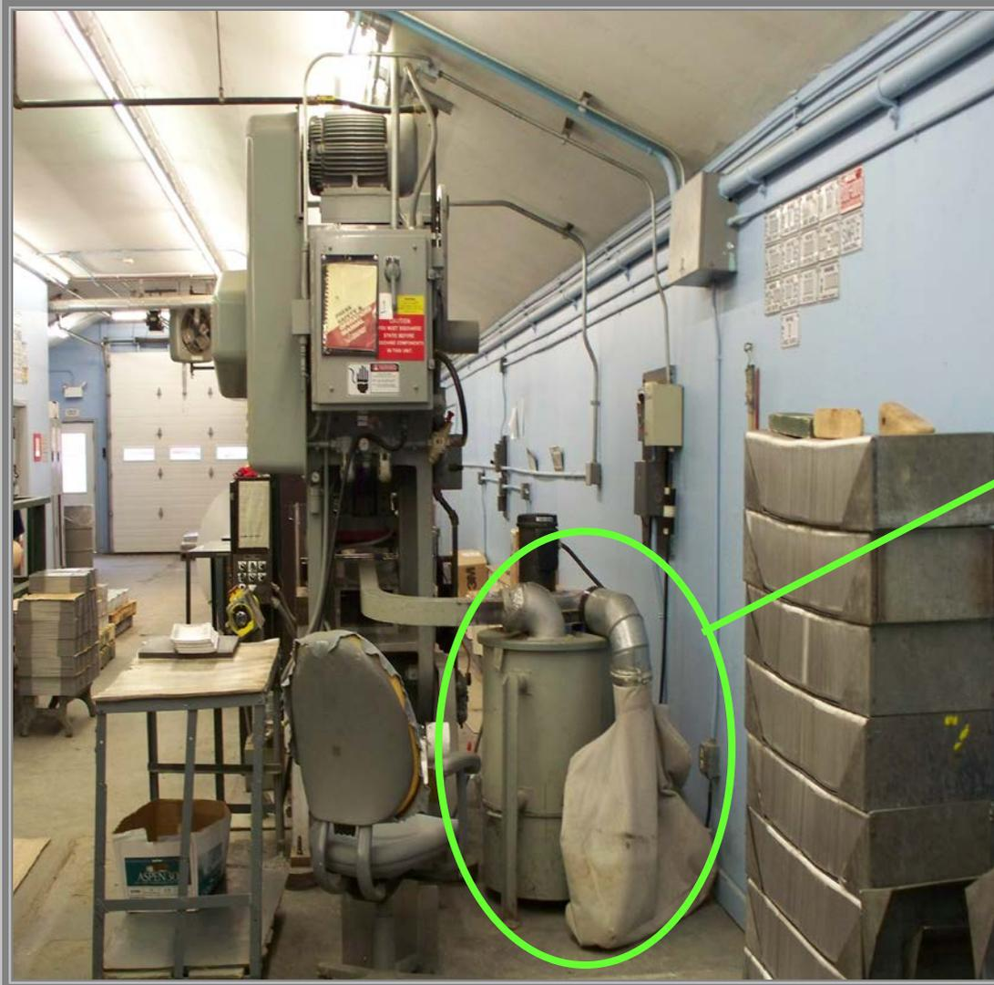
A view of the vacuum that collects the metal trimmings (corners and punched holes).
